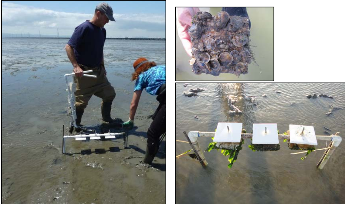
Figure 2. To assess recruitment to the sites, we used sets of tiles attached to frames at each of the study sites. The tiles were placed at the same tidal height and distance from shore as the restoration project at TNC, ELN and ELS. Tiles were first deployed in May 2012, and are removed and replaced quarterly. The standardized surface area of the tiles provides an ability to compare recruitment rates among the sites and between quarters.
