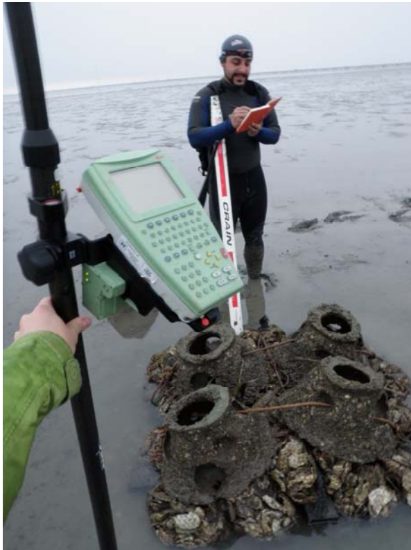
5. Collecting element elevations at Eden Landing Ecological Reserve site
