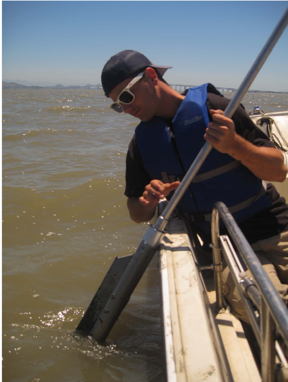
2. Collecting core at San Rafael site using a push-corer
