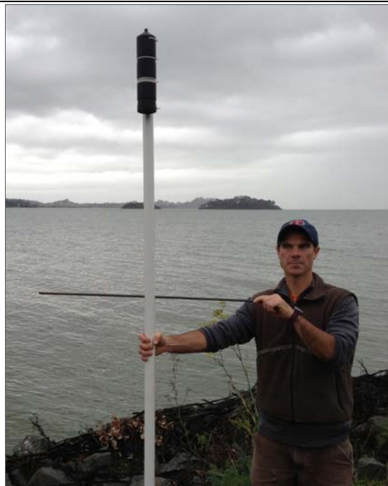
Photo 4 – Installation of a Vemco acoustic receiver at the TNC site.
